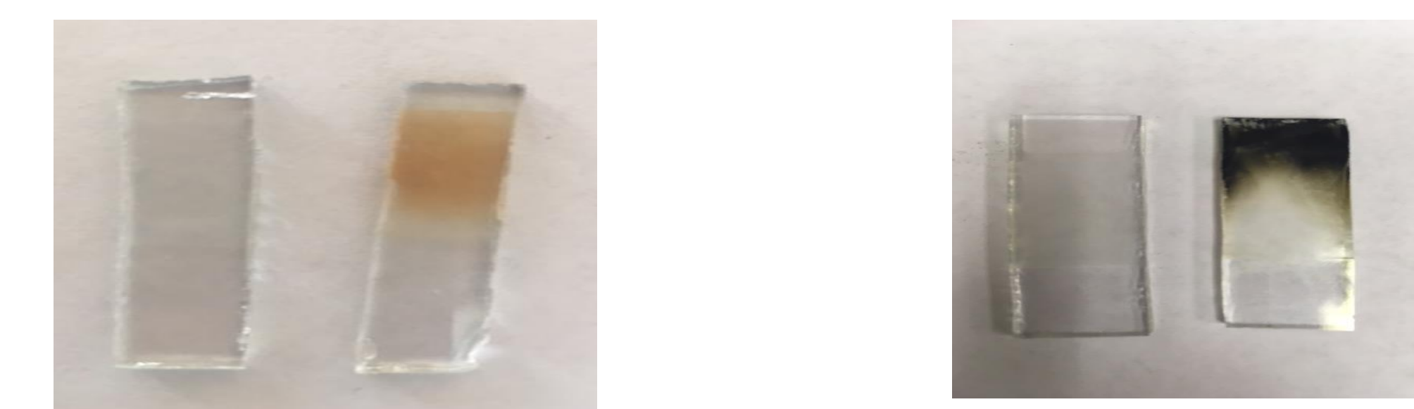
Picture 1. Titanium Oxide and Zirconium Oxide Semiconductors before and after photo electrolysis. In this experiment, the cell under white light illumination. This resulted in a what is suspected to be polymerization of Pyrene-1-Thiophene.
