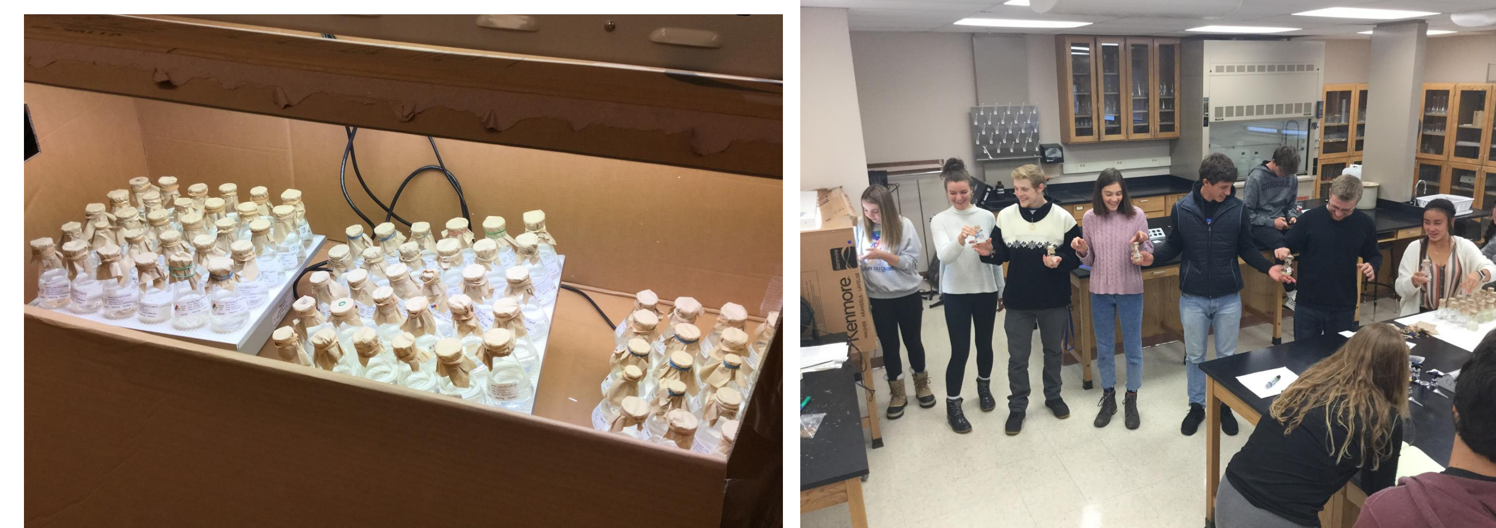
Figure 3. Algae cultivation occurred in a home-build grow chamber. The grow chamber was used to cultivate the algae. There was a 120 volts lamp that was on for 12 hours each day. The shaker tables were used to keep the beakers in motion to allow the algae to continue growing.
