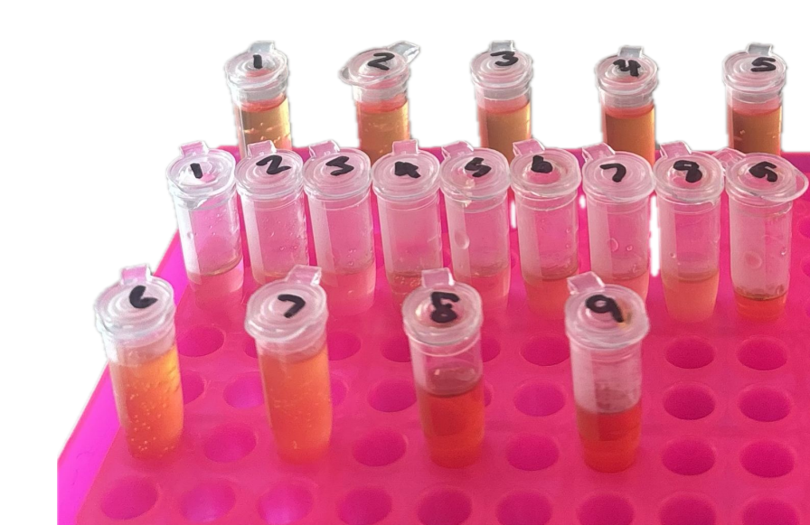
Figure 3. The TBARS Assay kit with urine samples from week two. In each sample, the color orange can be seen as a product of the 2-TBA reacting with ROS.
