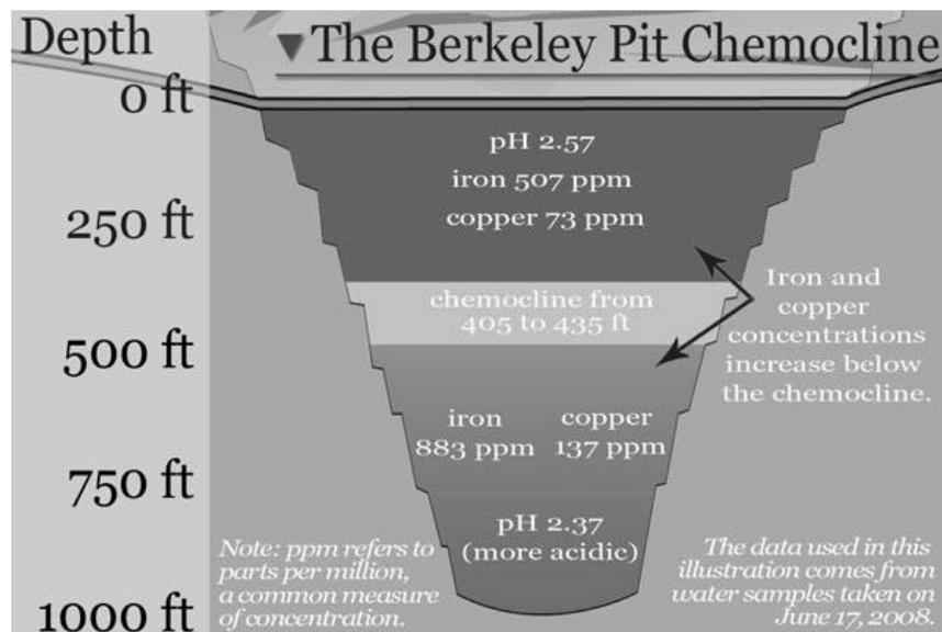
**Figure 2.** An animation of the epilimnion and hypolimnion of the Berkeley Pit. The chemocline, a zone of rapid chemical and physical change, separates stratified layers of the Berkeley Pit, allowing for two different pH levels and metal concentrations (image reprinted with permission, courtesy of "PitWatch").
