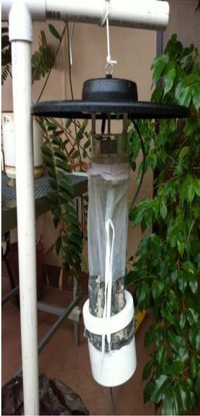
Figure 1: CDC Light Trap hood, mesh and container.
