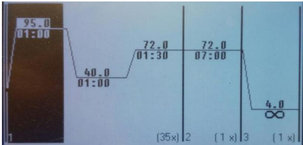
**Figure 2:** Folmer et al. (1994) thermocycler protocol. The x-axis represents time while the y-axis represents temperature in Celsius. The numbers above the line are the temperature settings for that period, while the numbers below represent the duration of the period. Vertical lines indicate sections where repeats occur, while the number in parenthesis indicates the number of repeats.
